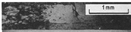
Figure 13 Optical micrograph of overall fracture topography of DGEBA-DETA (11 phr DETA) epoxy fractured at room-temperature at a strain rate of \sim 10^{-2} \text{ min}^{-1} .
